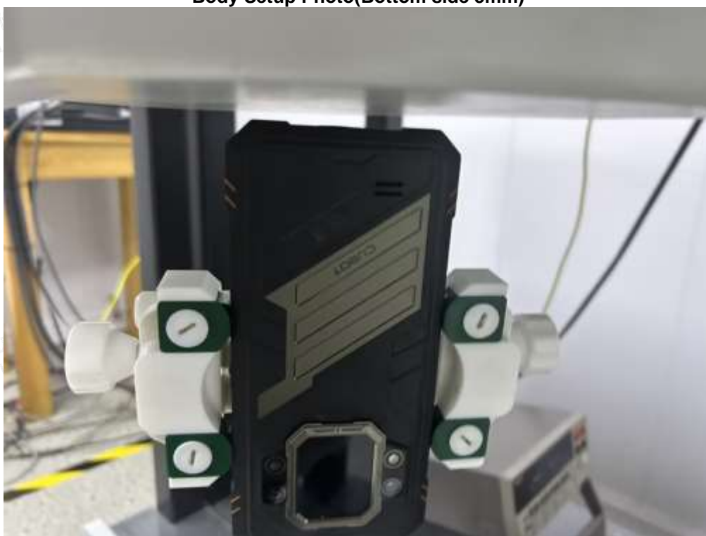
Body Setup Photo(Bottom side 5mm)
