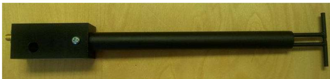
Figure 1 – MVG COMOSAR Validation Dipole
