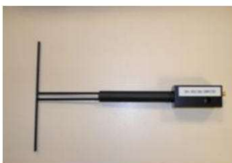
Figure 1 – Satimo COMOSAR Validation Dipole
