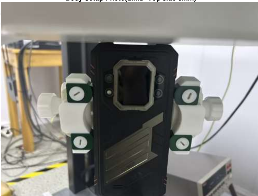
Body Setup Photo(Limb- Bottom side 0mm)
